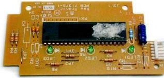
The microprocessor and controller circuitry of a keyboard.
