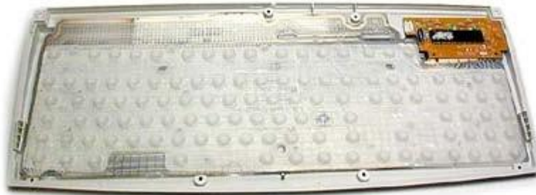
This keyboard uses rubber dome switches.
