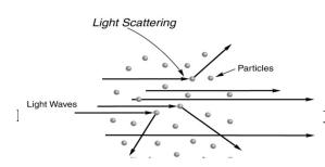
**Scattering:** scattering losses are caused by the interaction of light with
