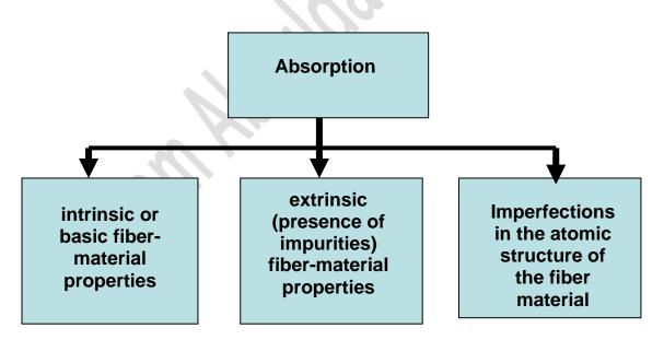
**Intrinsic Absorption**. Intrinsic absorption is caused by basic fiber-material properties. Intrinsic absorption sets the minimal level of absorption. In silica glass, the **wavelengths** of operation range from 700 nm to 1600 nm.
