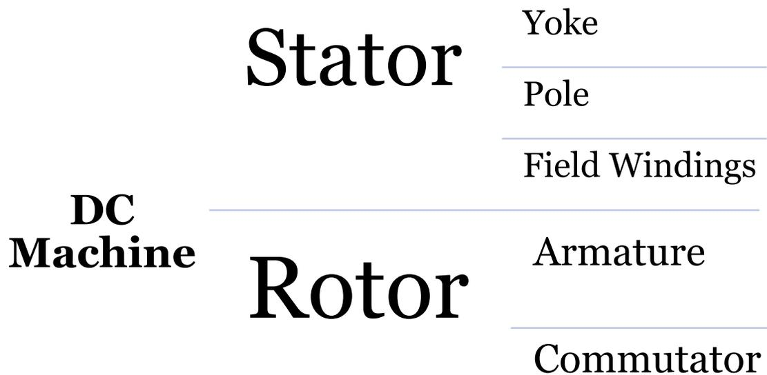
The essential parts of a DC machine are described below:
