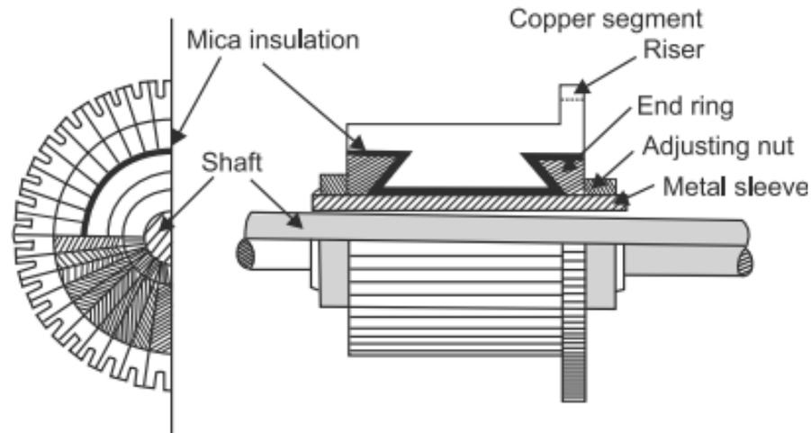
**Figure 8.** Commutator.
