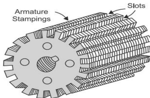
**Figure 6.** Armature core.
