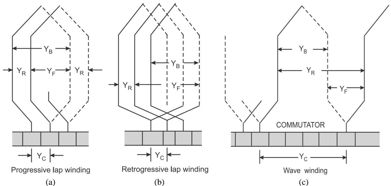
**Figure 13.** Terms used in coils.
