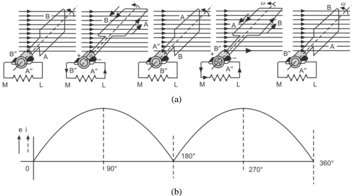
**Figure 10.** Generated emf for external circuit connected through split ring (a) Generated emf for external circuit connected through slip rings (b) Wave diagram.
