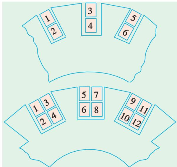
**Figure 14.** Double Layer Winding.
