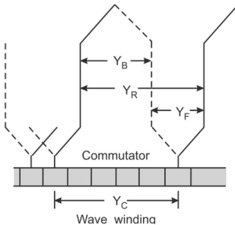
Figure 15. Wave winding.
