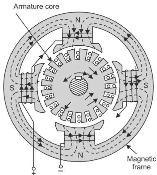
**Figure 5.** Magnetic circuit of DC machine.
