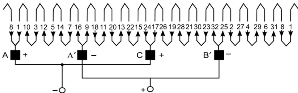
**Example 3:** Design a 4-pole, simplex lap winding suitable for an armature containing 20 slots. Assume single turn coils with 2 conductors per slot.
