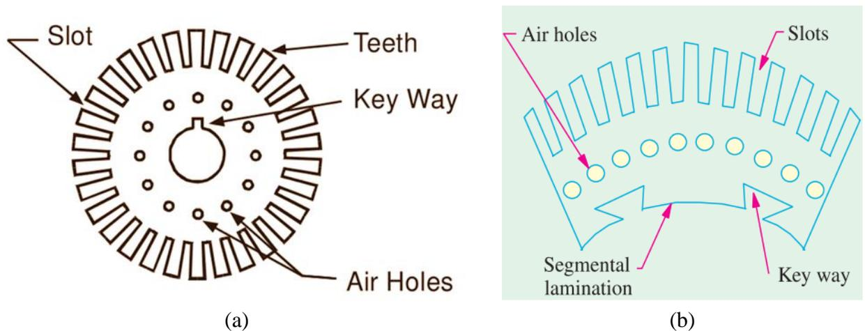
**Figure 7.** Armature core (a) Single circular lamination (b) segment.
