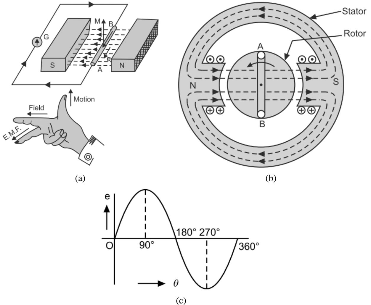
**Figure 2.** Generation of emf (a) Linear motion of conductor in a uniform magnetic field (b) Coil rotating in a uniform magnetic field (c) Wave shape of induced emf.
