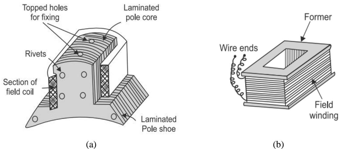
**Figure 4.** Pole core, pole shoe and field winding (a) Field winding placed around pole core (b) Field winding.
