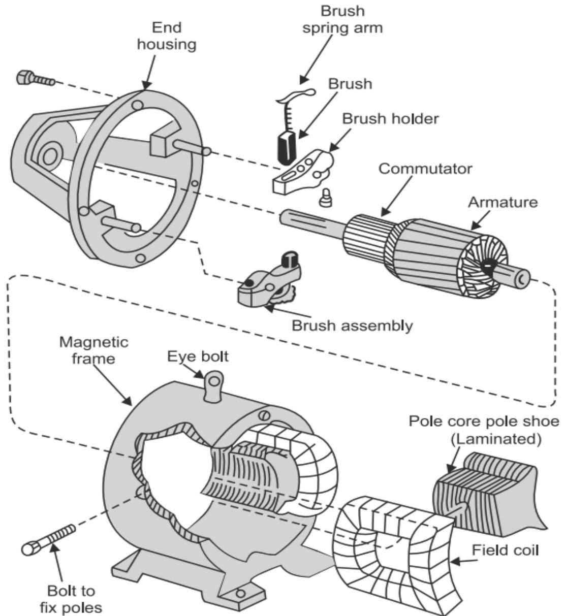
**Figure 3.** DC Machine Parts.
