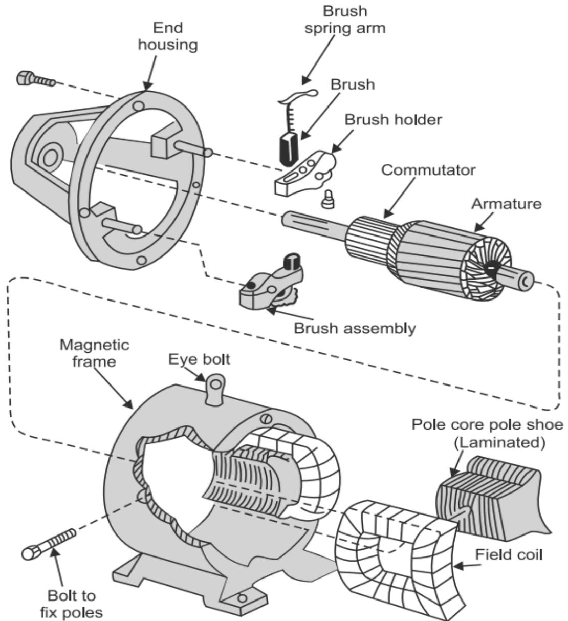
**Figure 3.** DC Machine Parts.
