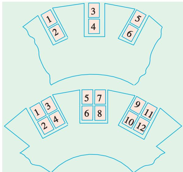
**Figure 14.** Double Layer Winding.
