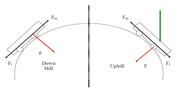
This operation is indicated as shown in the figure below in the first quadrant. Here the power flow is from the motor to load.
