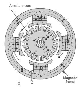
Figure 5. Magnetic circuit of DC machine.
