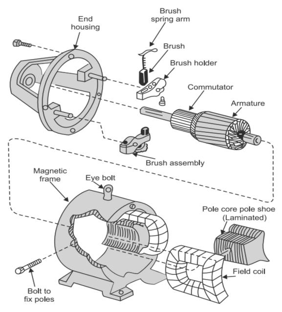
Figure 3. DC Machine Parts.
