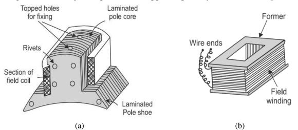
Figure 4. Pole core, pole shoe and field winding (a) Field winding placed around pole core (b) Field winding.
