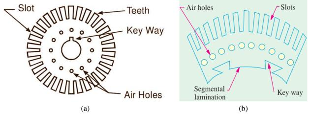
Figure 7. Armature core (a) Single circular lamination (b) segment.
