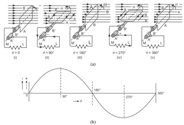
Figure 9. Generated emf for external circuit connected through slip rings (a) Load connected through slip-rings (b) Wave diagram.
