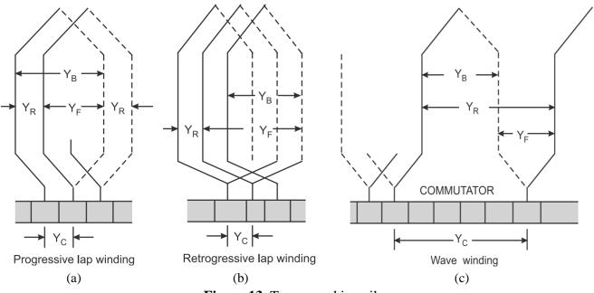
Figure 13. Terms used in coils.
