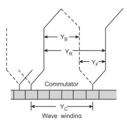
Figure 15. Wave winding.
