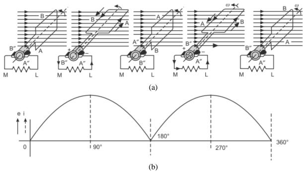
**Figure 10.** Generated emf for external circuit connected through split ring (a) Generated emf for external circuit connected through slip rings (b) Wave diagram.
