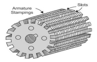
Figure 6. Armature core.
