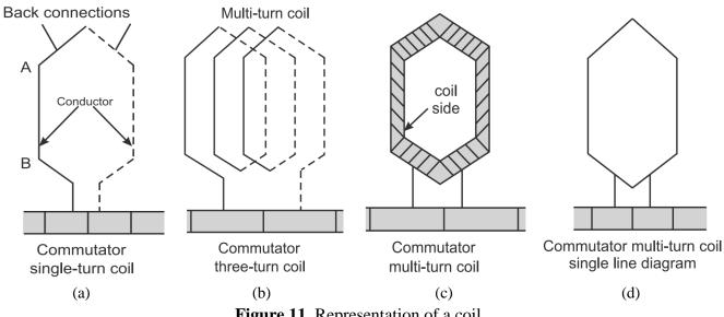
Figure 11. Representation of a coil.
