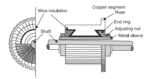
Figure 8. Commutator.
