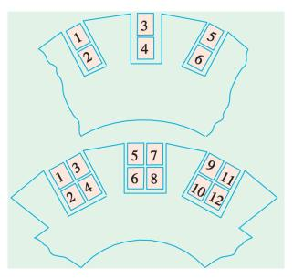
Figure 14. Double Layer Winding.
