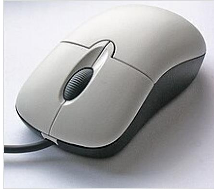
A computer mouse with the most common features: two buttons (left and right) and a scroll wheel (which can also function as a button when pressed inwards)
