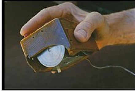
Inventor Douglas Engelbart holding the first computer mouse showing the wheels that make contact with the working surface
