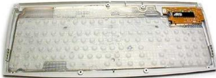
This keyboard uses rubber dome switches.
