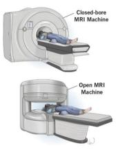
In MRI machines, the magnet is the main component responsible for generating a constant magnetic field, which forms the basis of the machine's physical function. The magnet creates a strong and steady magnetic field along the axis of the machine, called the primary magnetic field ( $B_0$ ). This field is the main factor that affects the protons in the human body, especially hydrogen protons, which are found in large amounts in water and fat in the body.
