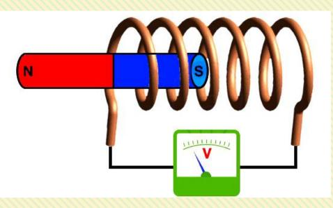
voltage in the loop. This voltage is proportional to the rate of change of the magnetic flux, leading to an induced current in the conductor.
