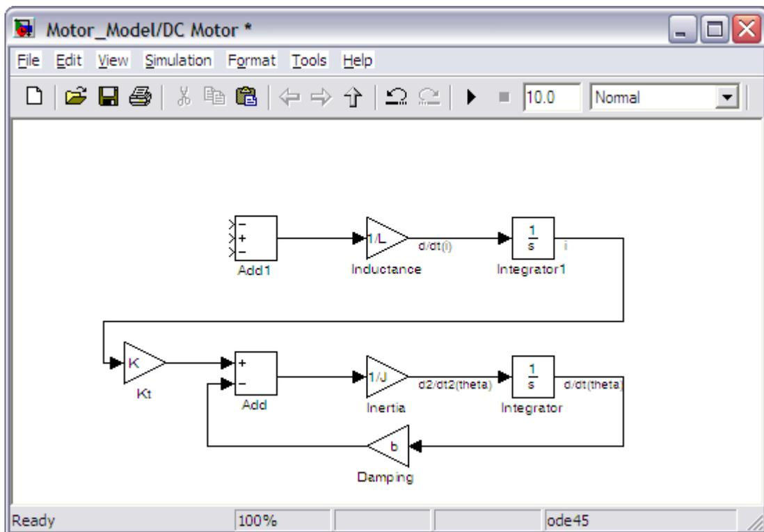
Now, we will add in the voltage terms which are represented in the electrical equation. First, we will add in the voltage drop across the armature resistance.
