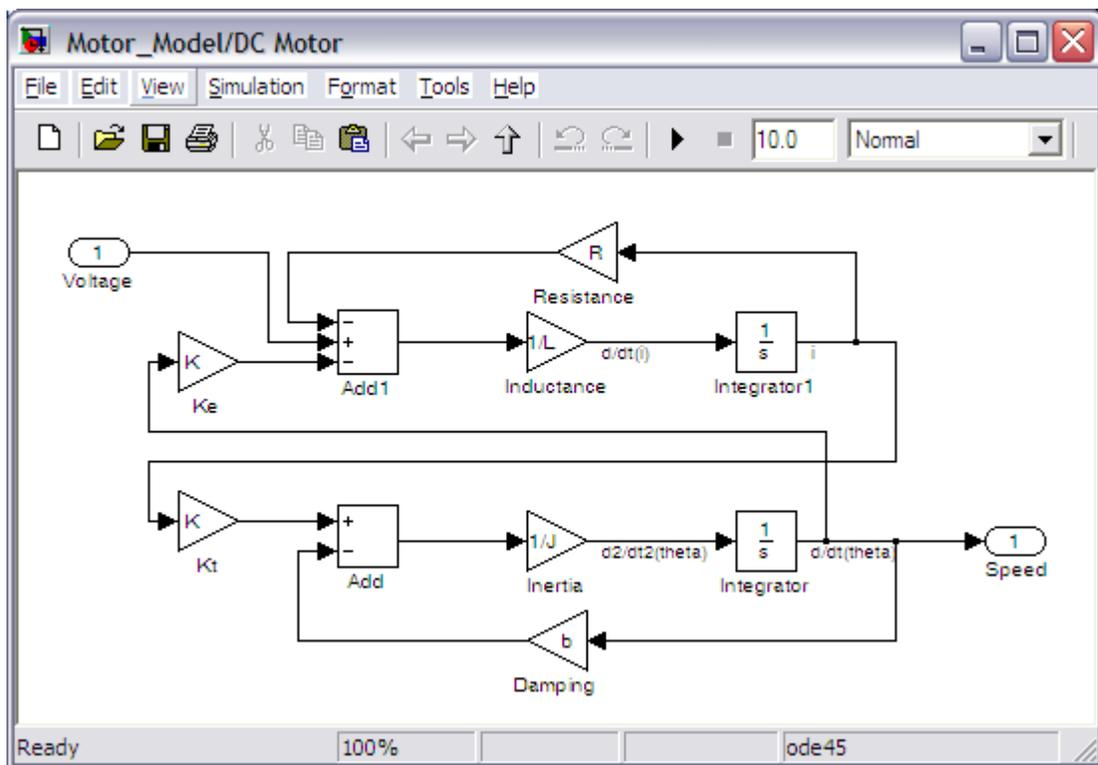
To save all of these components as a single subsystem block, first select all of the blocks, then select **Create Subsystem** from the **Edit** menu. Name the subsystem "DC Motor" and then save the model. Your model should appear as follows.
