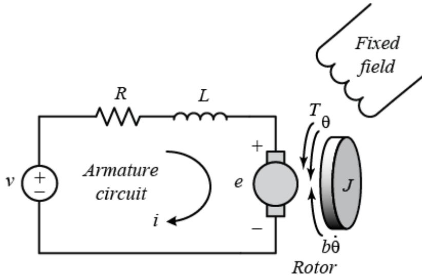
For this example, we will assume that the input of the system is the voltage source ( $V$ ) applied to the motor's armature, while the output is the rotational speed of the shaft  $d(\theta)/dt$ . The rotor and shaft are assumed to be rigid. We further consider a viscous friction model, that is, the friction torque is proportional to shaft angular velocity.
