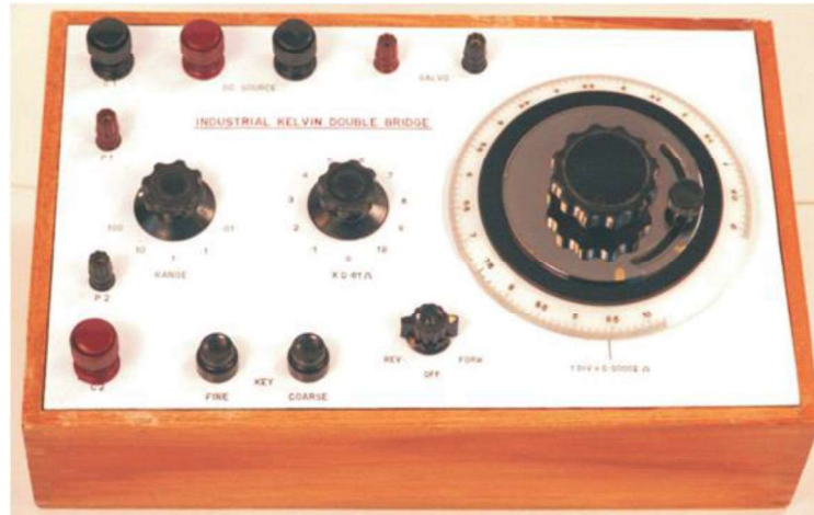
Fig. 4.8. Kelvin double bridge used in industry
