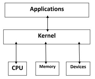
A kernel connects the application software to the hardware of a computer
