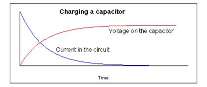
The product of the resistance and capacitance, RC, in the circuit is known as the time constant. This is a measure of how fast the capacitor will charge or discharge.
