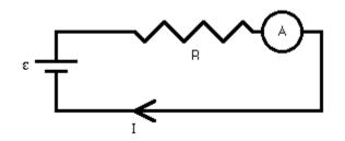
Remember that resistors in series have the same current flowing through them. An ammeter, then, must be placed in series with a resistor to measure the current through the resistor. On a circuit diagram, an ammeter is shown as an A in a circle. Again, the ammeter acts as a resistor, so to minimize its impact on the circuit it must have a small resistance relative to the resistance of the resistor whose current is being measured.
