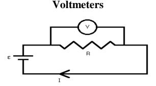
Resistors in parallel have the same voltage across them, so if you want to measure the voltage across a circuit element like a resistor, you place the voltmeter in parallel with the resistor. To prevent the
