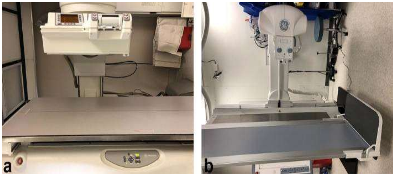
Figure (4): Shows two fluoroscopic imaging equipment: (a) A standard fluoroscopic machine with a 45 cm aperture opening, (b) Bariatric fluoroscopic machine with 63 cm aperture opening.
