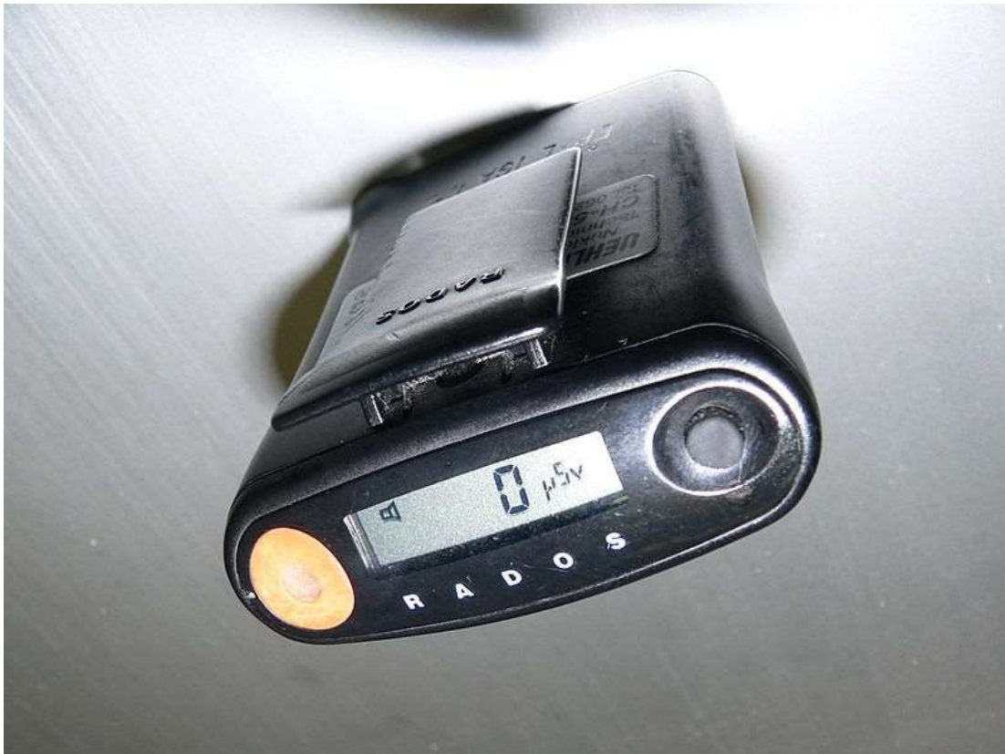
Figure (7): Shows a view of the readout on an electronic personal dosimeter. The clip is used to attach it to the wearer's clothing.
