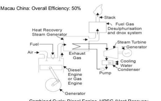
Combined Cycle: Diesel Engine, HRSG (Heat Recovery Stream Generator) and Steam Turbine. **Example 1.** A diesel power station has fuel consumption of 0.28 kg per kWh, the calorific value of fuel being 10,000 kcal/kg. Determine (i) the overall efficiency, and (ii) efficiency of the engine if alternator efficiency is 95%.
